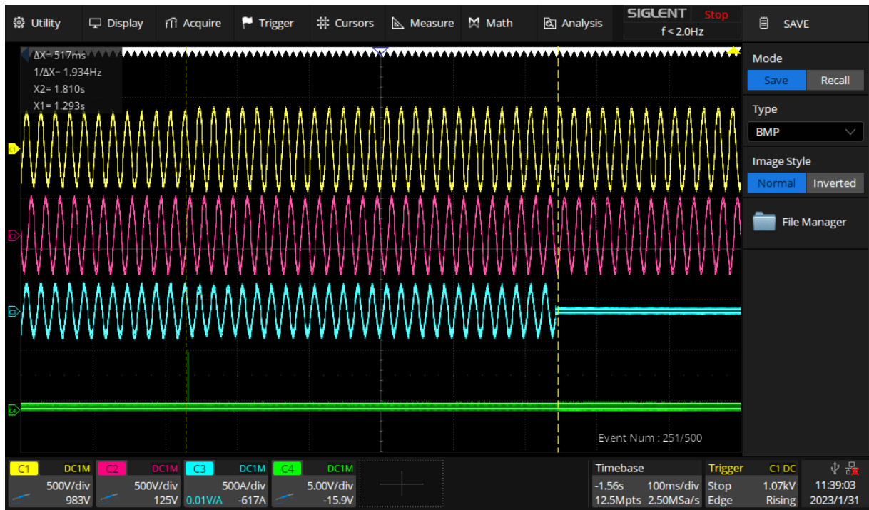
Figure 17 – Test O/V stage 2 (Trip test, L3-N)
