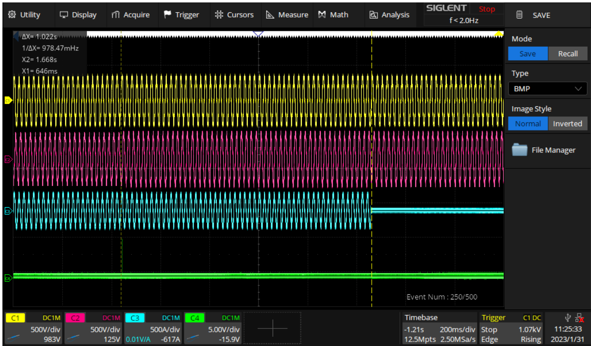
Figure 13 – Test O/V stage 1 (Trip test, L2-N)
