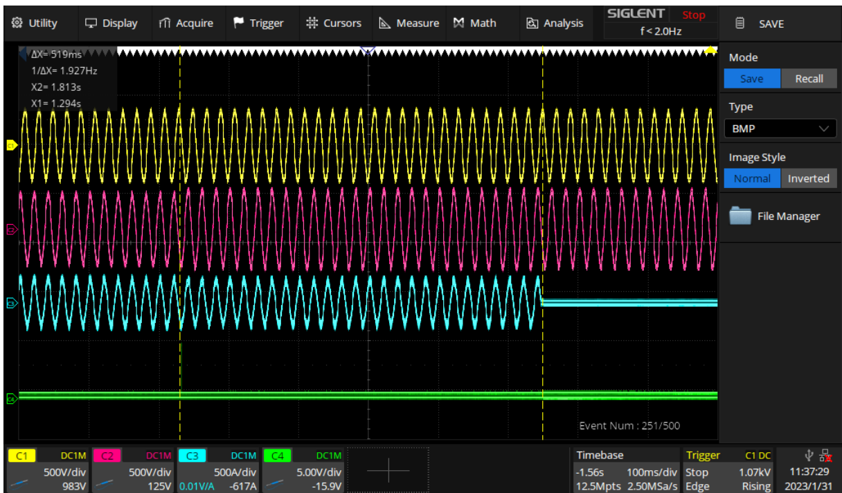
Figure 16 – Test O/V stage 2 (Trip test, L2-N)
