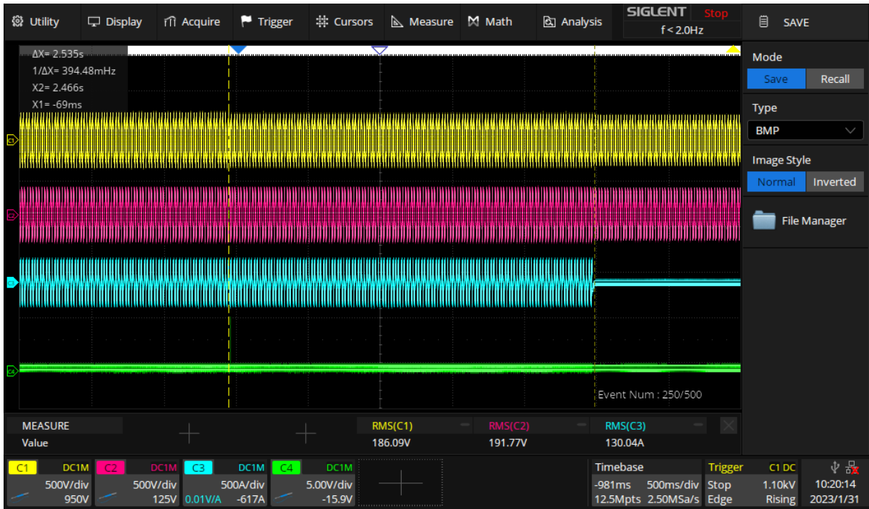
Figure 11 – Test U/V (Trip test, L3-N)
